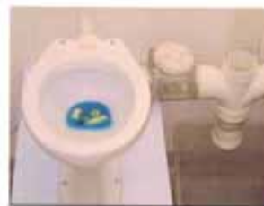
Figure 4. Setup for Solid Waste Flushing Characteristics Test
