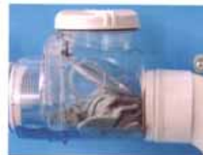
Figure 5. Setup for Bulky Foreign Matter Passage Test
